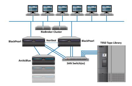
In Spectra RioBroker's multi-node cluster configuration, data mover nodes failover automatically to each other including database replication/sharding and job queue. Failover is seamless and allows redundancy without extra overhead. Furthermore, behind a cluster of Spectra RioBrokers, BlackPearl can also be set up as a hot-pair system, allowing automatic failover of the object storage controller. Normally, however, data replication to a second BlackPearl,
