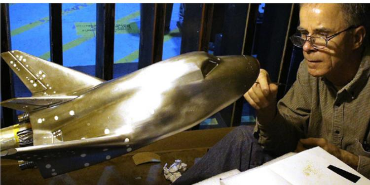
NASA technician Ricky Hall works inside the Unitary Plan Wind Tunnel at NASA's Langley Research Center in Virginia to affix grains of sand to a precise scale model of the Dream Chaser spacecraft. The sand creates turbulence at key points to simulate the conditions the real spacecraft will encounter during its return to Earth. The data gathered from the wind tunnel was used to further test the design through the company's Commercial Crew Integrated Capability agreement with NASA.
