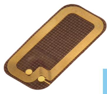
Each piece of tape media is equipped with a Media Auxiliary Memory (MAM) chip, which is embedded by the manufacturer. The MAM chip serves as a storage unit for small amounts of data and can transmit this information over RFID, making it a key component in data management.
