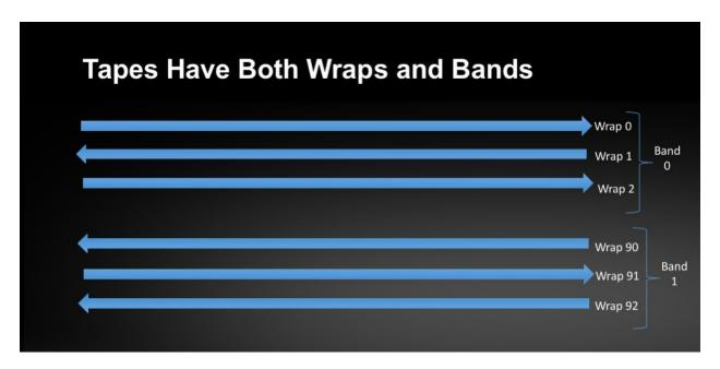
Due to the out and back way files are written to tape, retrieving files in their logical sequential order is one of the least efficient methods of reading files.
