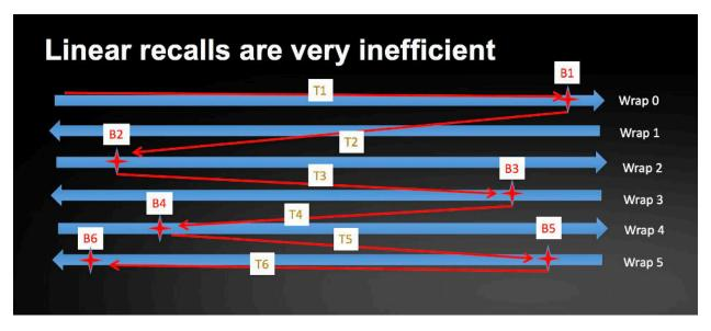
This is a result of locating up and down the tape unnecessarily with a maximum penalty of traversing 970 meters to get to the next file.
