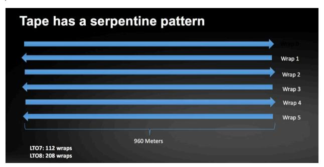
In addition, the tape head only covers about a fourth of the width of the tape so it needs to be moved to one of four positions. These four positions are known as bands. So, for LTO-8 tape, there are four bands each consisting of 52 wraps. Moving between wraps contained within a band is faster than moving to a wrap on another band. Also moving to a wrap that is in the same direction is faster than moving to one that is in the opposite direction.
